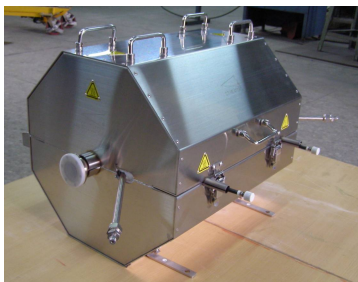
BURNING CHAMBER (maximum temperature 900°C)
