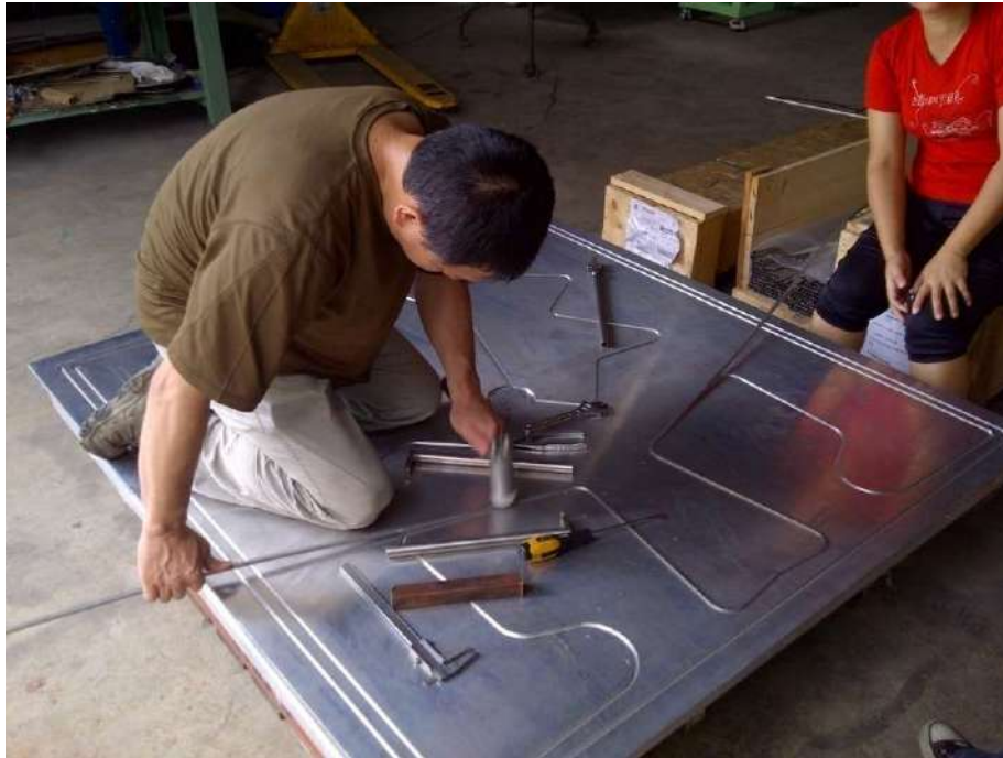
5.7G susceptor during the process Heating elements bending formation
