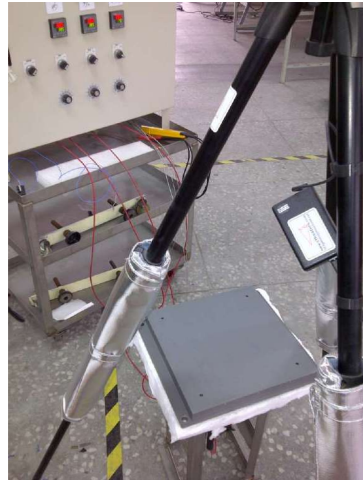
AL, hard anodized 2 heating zones, dim. 350X310X40T mm, 220V 1.8kW (outer zone), 220V 1.2kW (inner zone)
