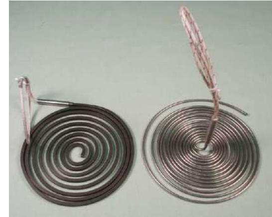
EXAMPLE OF VACUUM PUMP HEATING ELEMENTS
