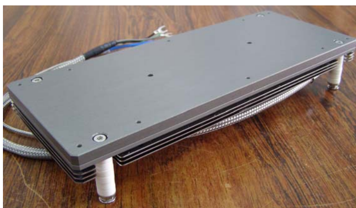
220V800W w/ K-type sheath thermocouple Hard anodized aluminum, dim: 270X105X10T mm
